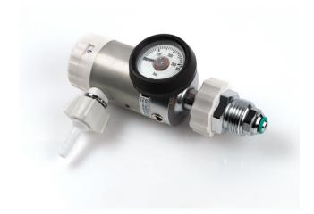
The **JUST Press P** for **REANIVAC** is a compact oxygen regulator that incorporates a dial dlowmeter. It can be connected to all of the officially aproved cylinder sizes and it integrates a pressure gauge for pressure measurement.
